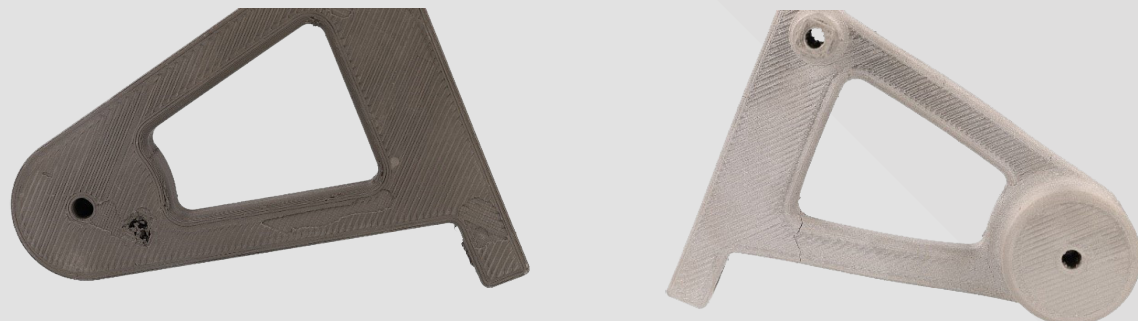
Figure 16: Damaged Bottom Surface and Resulting Top Cracks
