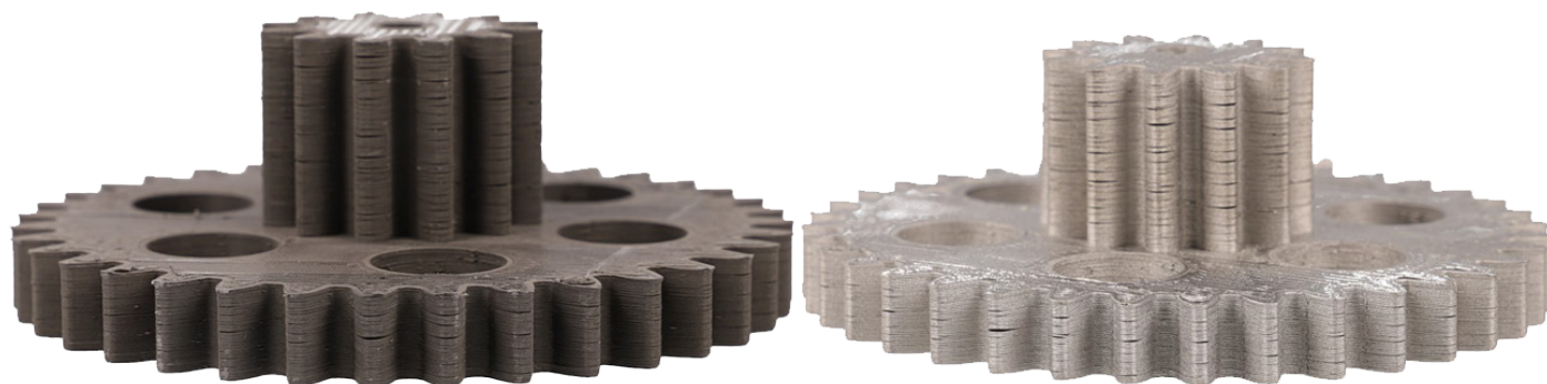
Figure 6: Print Delamination Become Sintered Cracks
